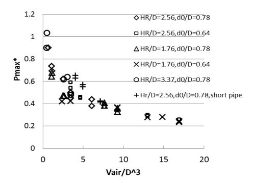
Figure 8: Measured maximum pressures for various experimental configurations and air volumes.
