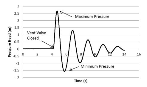
Figure 7: Typical pressure transient.
