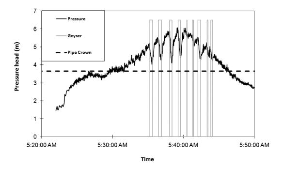
Figure 2: Title of pressure measurement during geyser episode in Minneapolis, Minnesota stormwater system. Gray lines depict the times during which geysers are visible on videotape (no scale). Dashed line depicts pipe crown, flow is surcharged when pressure is above pipe crown.
