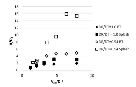
Figure 5. Rise heights for two different riser diameters (riser diameter/tunnel diameter of 0.54 and 1.0)
