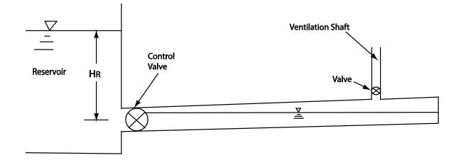
Figure 6: Schematic of experimental apparatus to measure pressure transients due to air compression against an advancing hydraulic bore.
