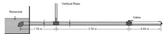
Figure 3: Schematic of experimental apparatus to observe water displacement in vertical riser by air pocket.
